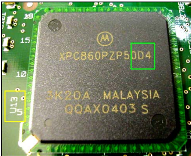
Figure 6. 1721: Compliant Motorola processor, with “D” revision.
