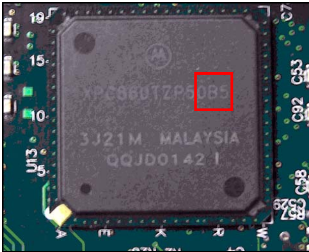
Figure 5. 1721: Non-compliant version ‘B’ Motorola processor.
